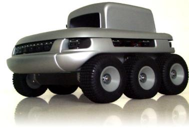
In addition to this, the robot retains the structure and is compatible with the smaller Khepera robot permitting programs and experiments to be migrated between the two. It also features 16 infra-red and ambient light sensors arranged around the robot in all directions, especially focused on the front.
